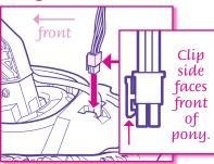
Snap in electrical connector clip from head into body. Make sure clip side of connector faces toward front of pony.
